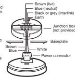
If desired, the alarm can be interconnected with up to 11 other smoke (SW1), heat (HW1) or carbon monoxide (CW1) alarms from the FireAngel range via the 'I' connector. (See Optional Interconnecting Feature).
